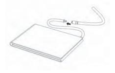
Connect the air hose to the NIBP connector on the Super Unit.
