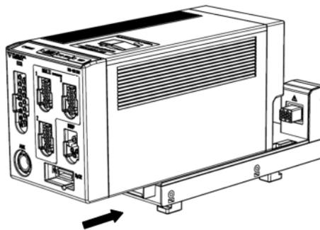
The HS-8000 can be connected/disconnected from the HSA-80 with the main unit power turned ON.
