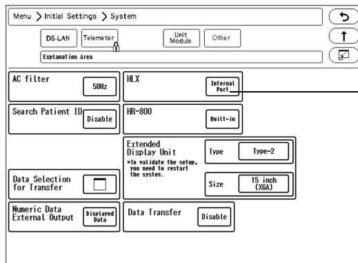
**2** If the HLX-801 (FA) / HLX-801 (G) is installed in the internal slot, select [Internal Port].
