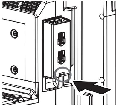
**□ Removing the Expansion Module**
