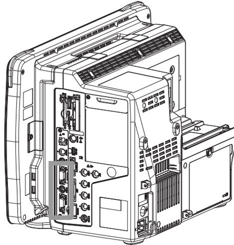
The above illustration is when the optional CC-84 Expansion Board is installed. .
