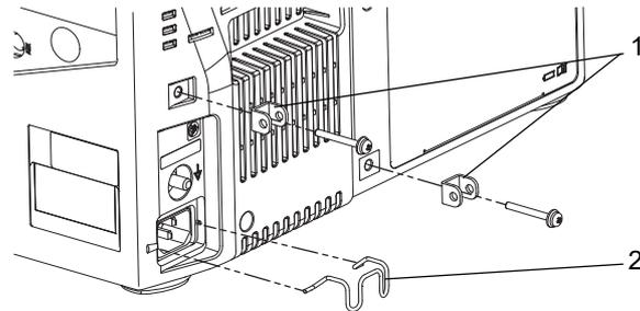
**2** Connect the power supply cable to the main unit.
