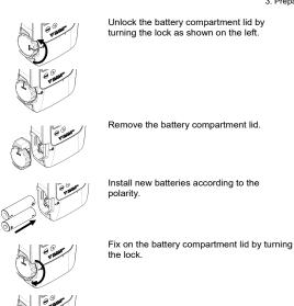
Make sure that any foreign particles, such as hairs, are not held on the battery compartment lid and dust is not adhered to the edge of the lid to prevent water entering into the battery compartment area.
