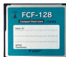
FCF-128 (1Z7333B) 128MB CF Card Flash Memory Card *for transferring monitor settings
